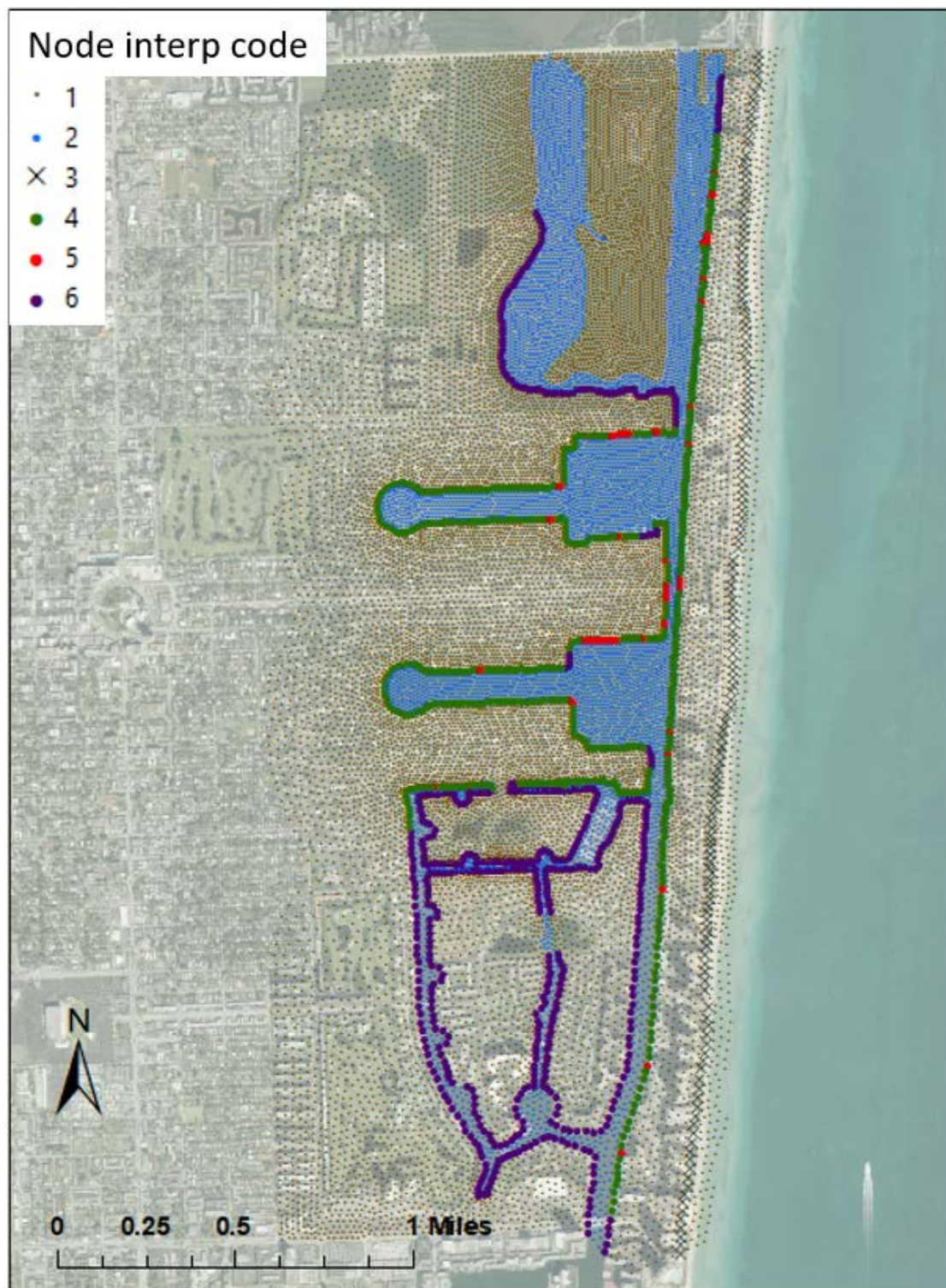
Figure 2.12 Mesh Node Elevation Interpolation Codes, Hollywood Lakes
